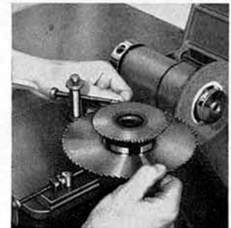
SAW GRINDING and TRUING DEVICE — a rapid and precise means of both grinding and truing blades. Truing is automatically done at the same time as grinding through the use of a master index plate. It is particularly convenient with All-Purpose Blades which are ground only and not swaged.
