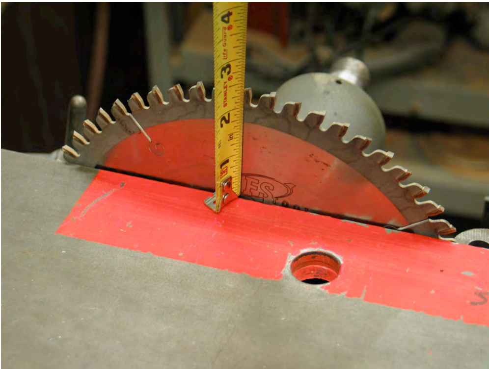
Figure 335 Cutting height with the new arbor will be slightly shy of 2-1/2 inches, a very acceptable range for a saw this small.
