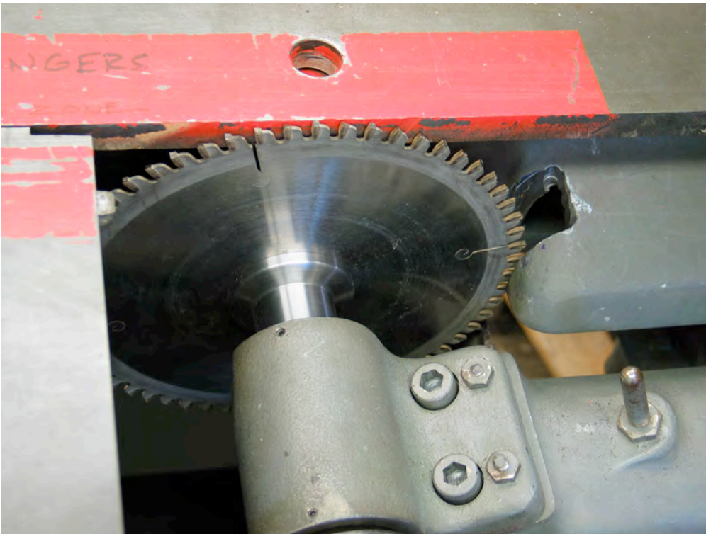
Figure 357 The installed blade ready to go.
