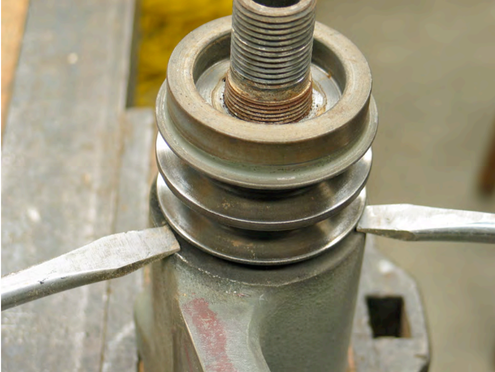
Figure 12 Pry off pulley with a couple of screwdrivers. Remember, there is a woodruff key under the pulley.
