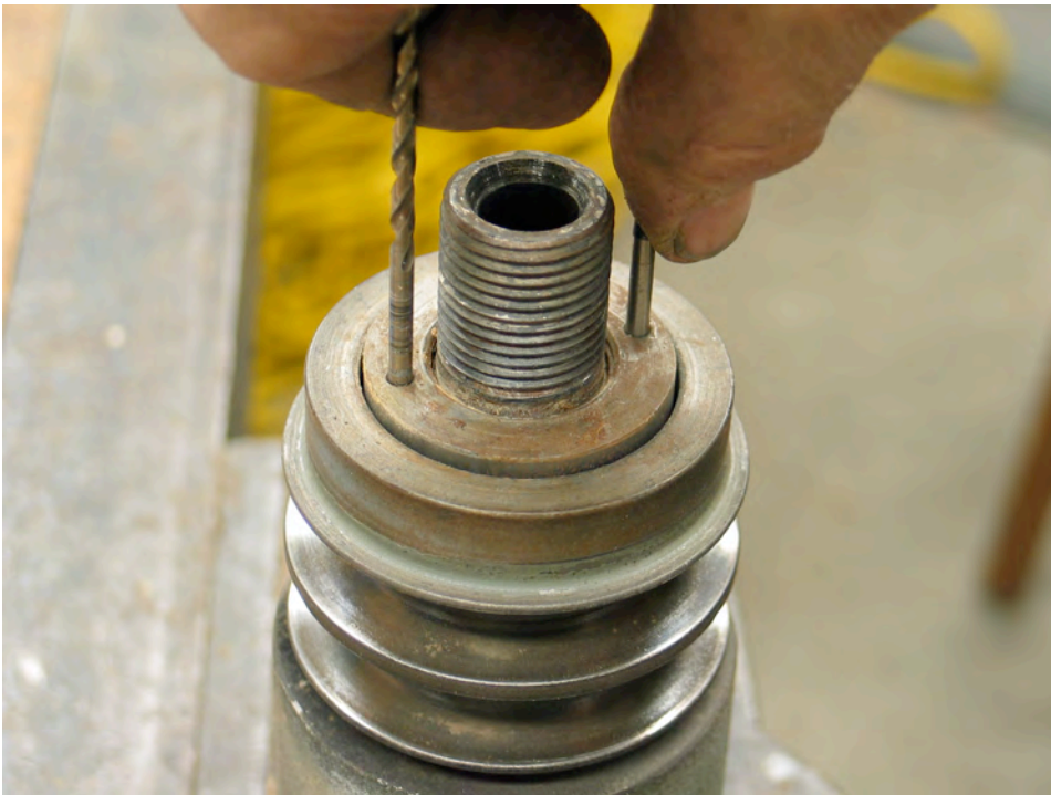
Figure 11 Once the spanner nut is loose, remove with hands.
