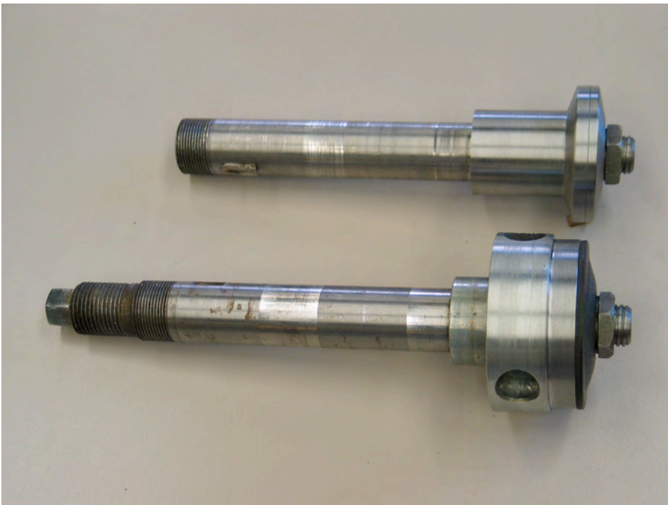
Figure 2921 For comparison, the top shaft is the new one and the bottom one is the faceplate style. Note the different dimensions around the flange.
