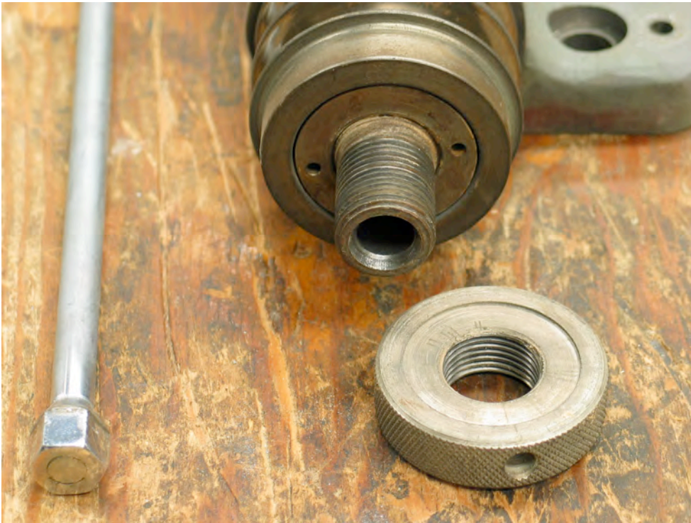
Figure 7 Auxiliary threaded ring removed to expose spanner nut that holds the pulley against the bearing. The auxiliary threaded ring will be discarded.
