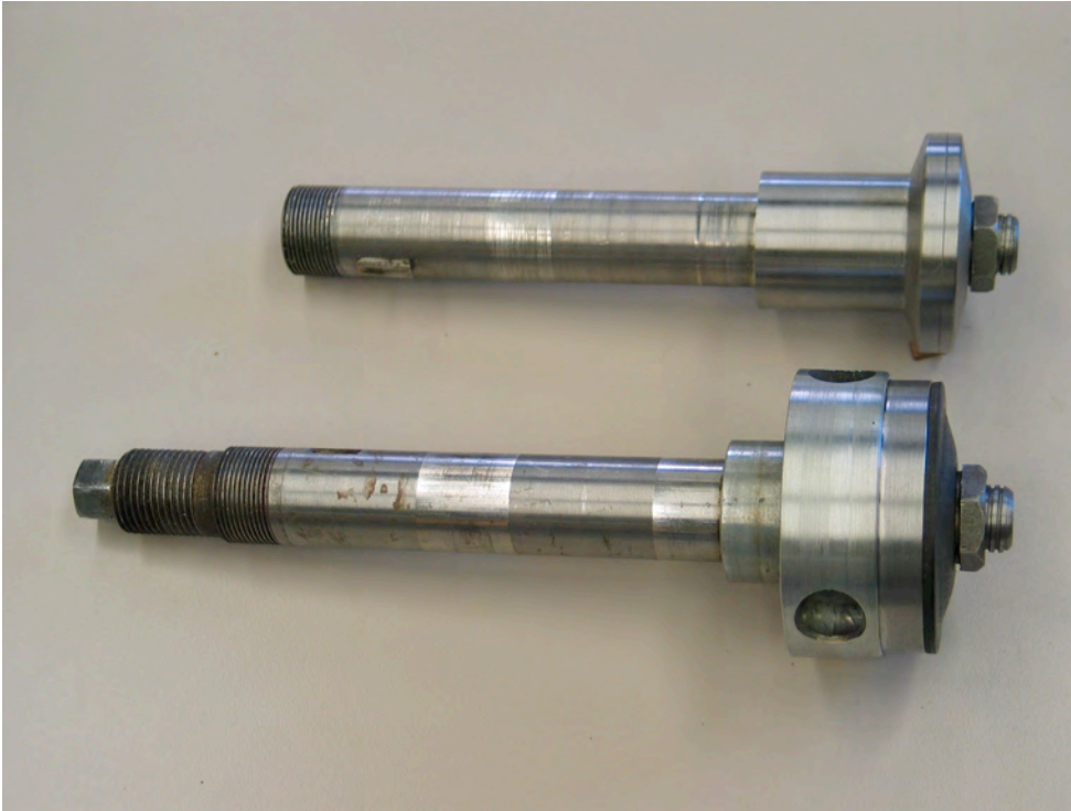
Figure 24 Here's two approaches to a solution. Both use a Unisaw LH nut. The top shaft is newly made with a smaller blade flange (2-1/4"). The lower flange uses a newly made face plate held in with the original drawbar.
