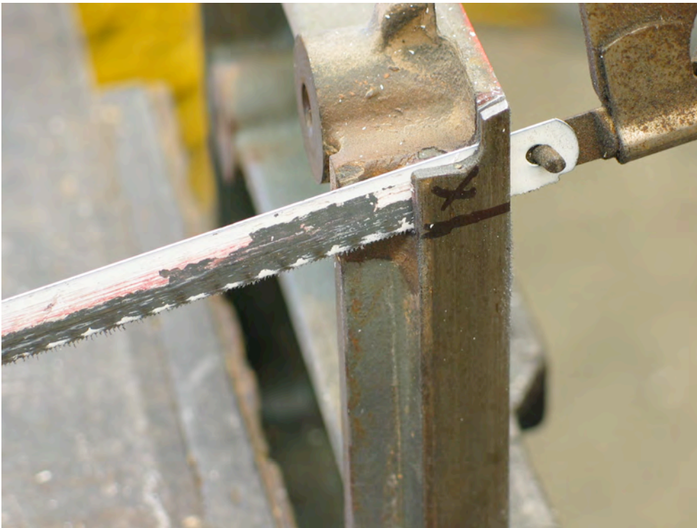
Figure 21 A hacksaw makes quick work of this detail.
