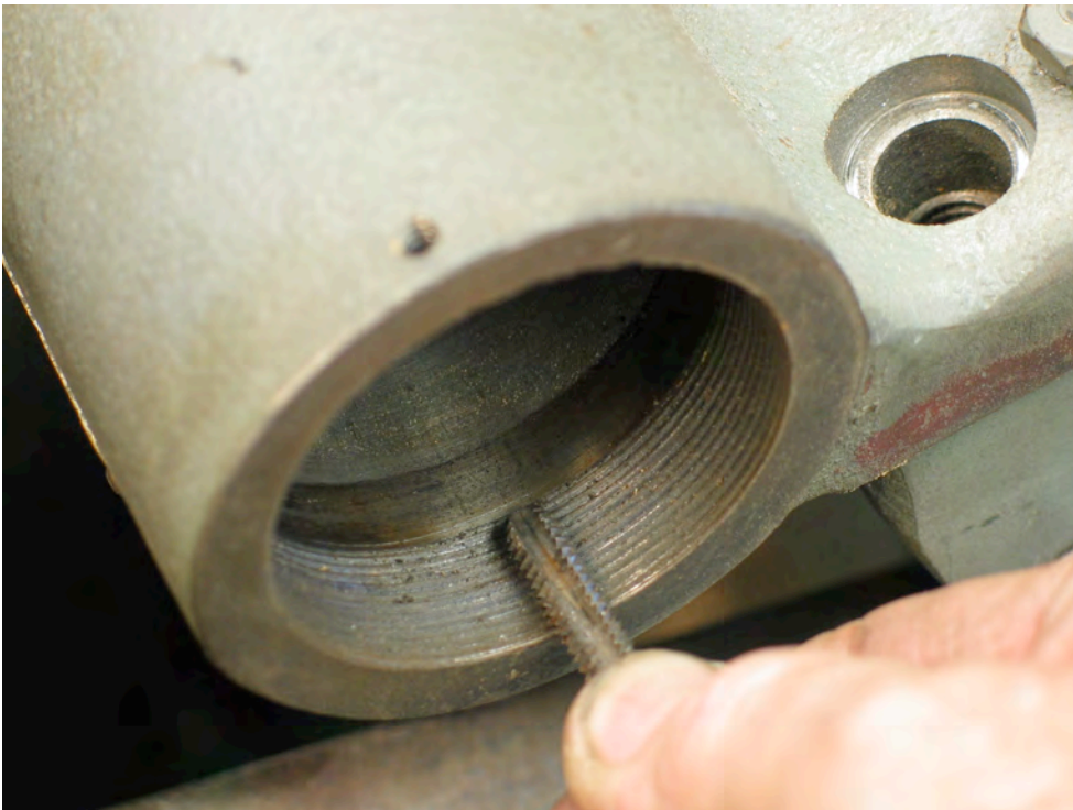
Figure 23 Clean the threads with a 1/4-20 tap so the spanner nuts will install easily.
