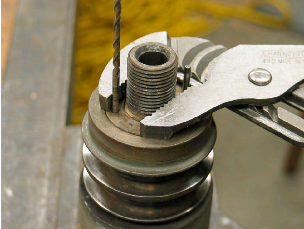
Figure 10 To break the friction, install a couple of 1/8 inch pins as studs and twist if you don't have the right size spanner wrench.
