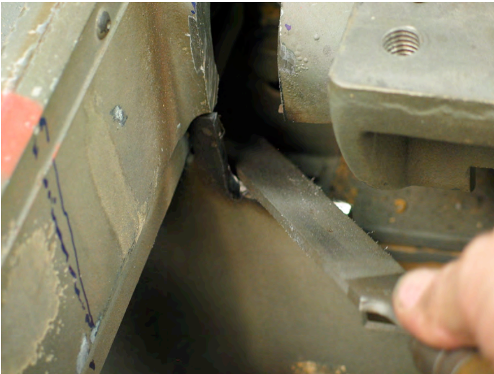
Figure 313 A little work with the file cleans up the edge.
