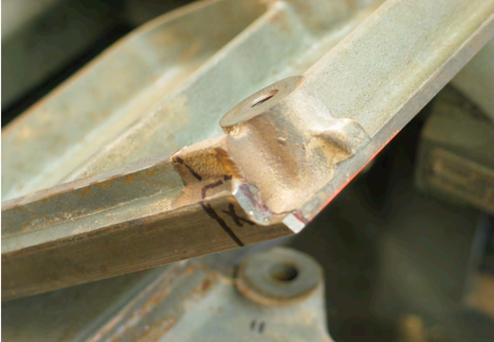
Figure 20 Table is removed after the cut area is marked
