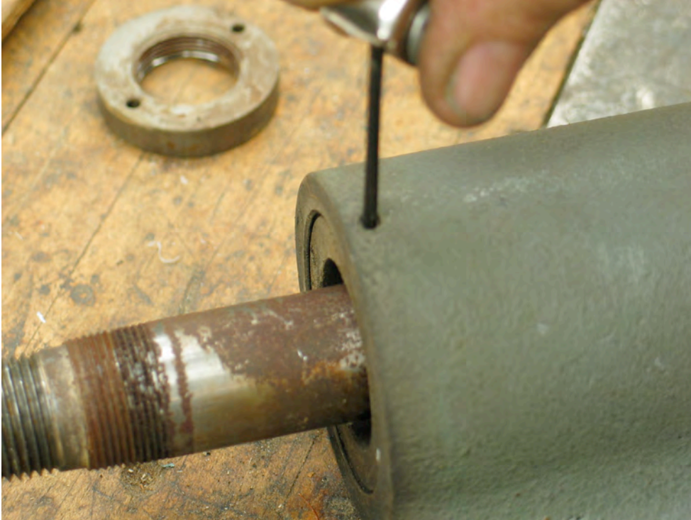
Figure 8 remove the two setscrews that hold the bearing retaining rings. Be careful to keep the brass compression stud under the setscrews.
