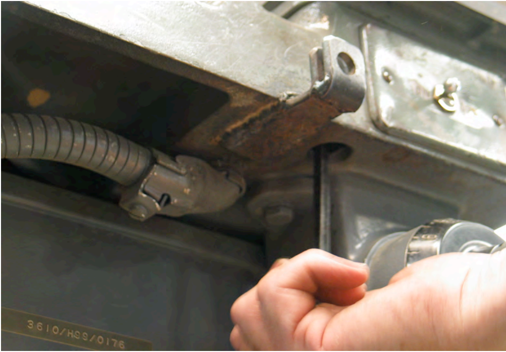
Figure 16 Now that the top is out, the table needs to be removed by removing three socket-head cap screws
