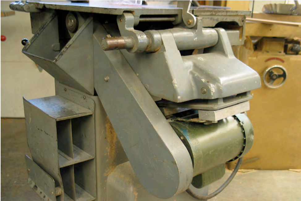
Figure 50 side view of the new motor installation.
