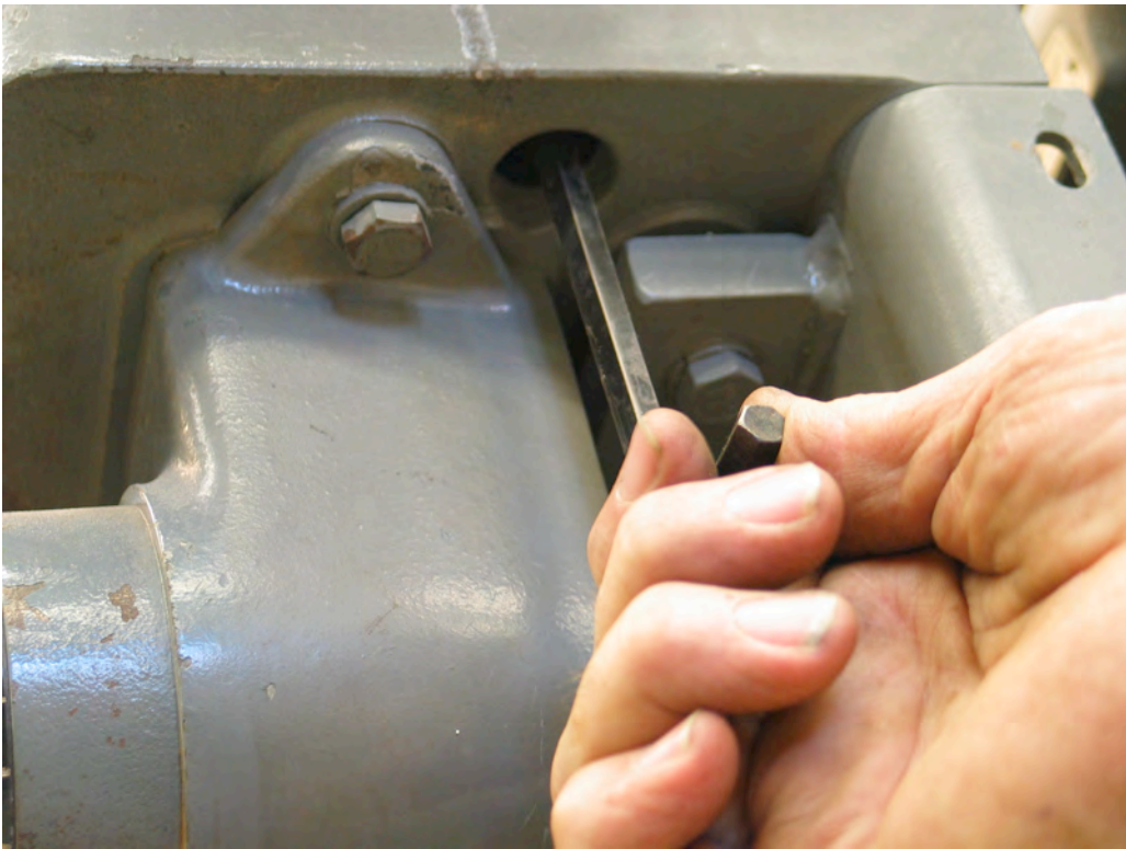
Figure 17 Like the first cap screw, access to the second is through a hole in the casting
